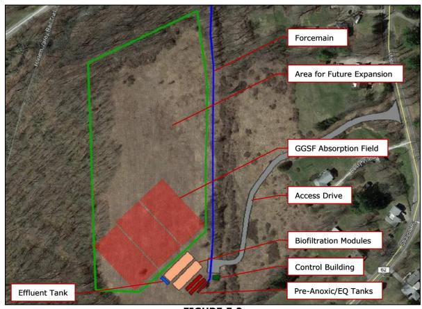
**FIGURE 5.2** Preliminary Layout of Alternative No. 2
