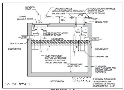
**FIGURE 4.2** Typical Septic Tank
