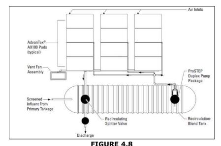
Typical Orenco AdvanTex System Layout for Subsurface Disposal
