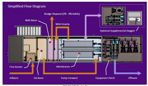
**FIGURE 4.6**Ovivo MicroBLOX Simplified Process Flow Diagram
