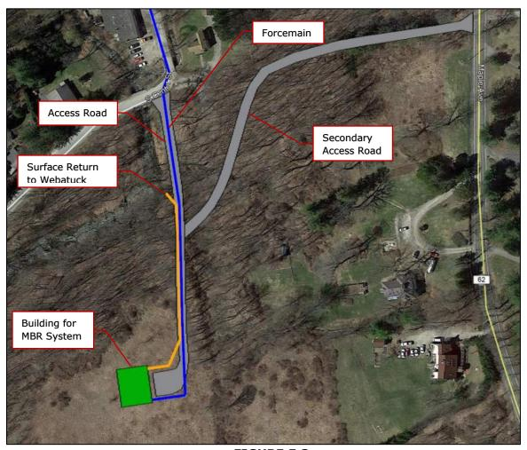
**FIGURE 5.3** Preliminary Layout of Alternative No. 3
