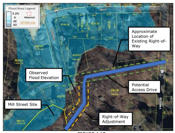
**FIGURE 4.17**Approximate Right-of-Way Location at the Mill Street Site
